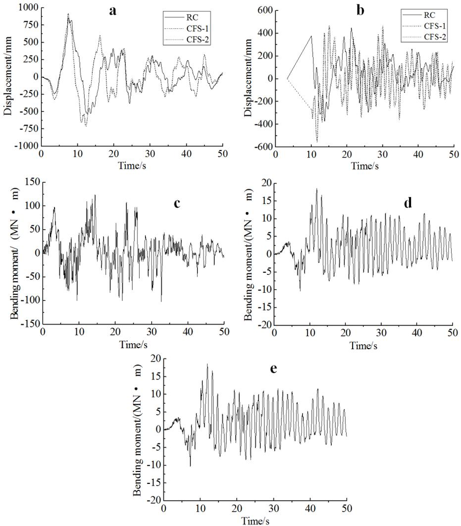
Fig. 5. Displacement time-history and bending moment time-history curves: **a**—PGA is 1.2 g at pier's top, **b**—PGA is 1.2 g at pier's middle height, **c**—PGA is 1.2 g (RC pier), **d**—PGA is 1.2 g (CFS-1 pier), **e**—PGA is 1.2 g (CFS-2 pier)
