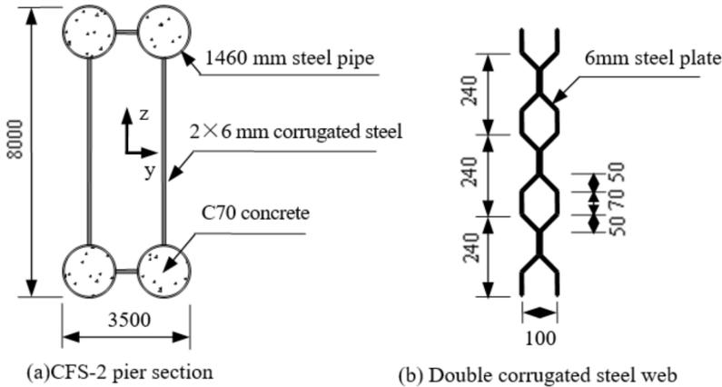
Fig. 4. CFS-2 pier section (dimensions in mm)
