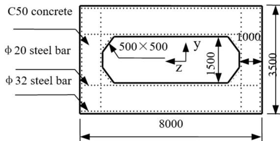
Fig. 2. Layout of main bridge (dimensions in mm)
