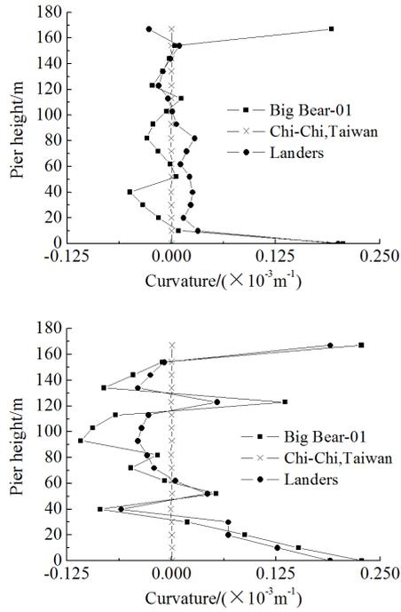
Fig. 6. Maximum curvature envelope of pier along the high direction of the pier:
