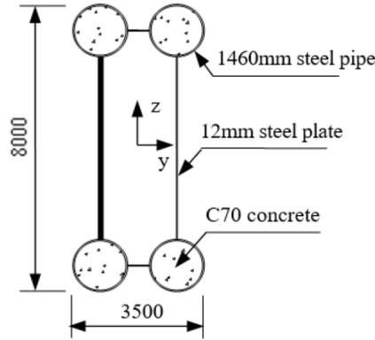
Fig. 3. CFS-1 pier section (dimensions in mm)
